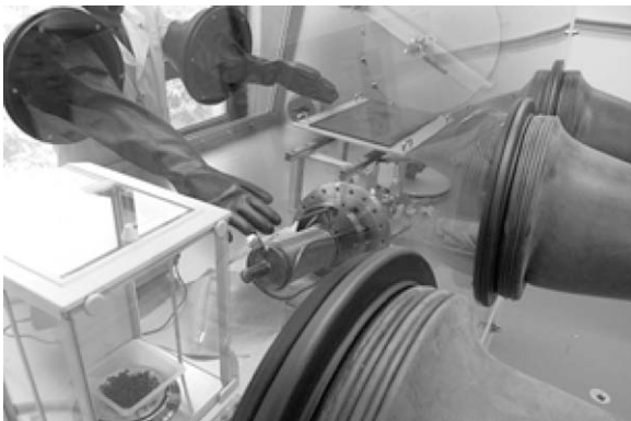
Fig. 2. Metal hydride bed in the glovebox.
