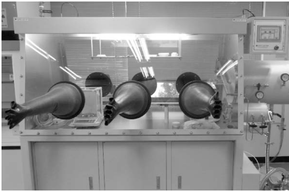
Fig. 1. Glovebox for the metal hydride bed preparation.
